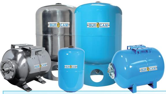
Replaceable bladder. Made of Butyl rubber to increase reliability and life span. Tough, epoxy-baked or stainless steel finish. Pressure: Tested to 150 PSI. Maximum operation pressure of 75 PSI. Flange made from stainless steel. Factory pre-charged at 28 PSI.
