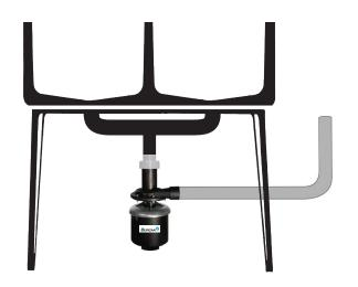
For installation on a twin laundry tub, the pump has to be centered as per this diagram.
