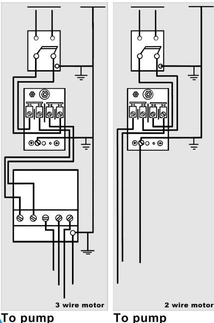
Pressure switch setting (start/stop 20/40 or 30/50)has been made in factory. An adjustment may be done to give other operating pressures.
