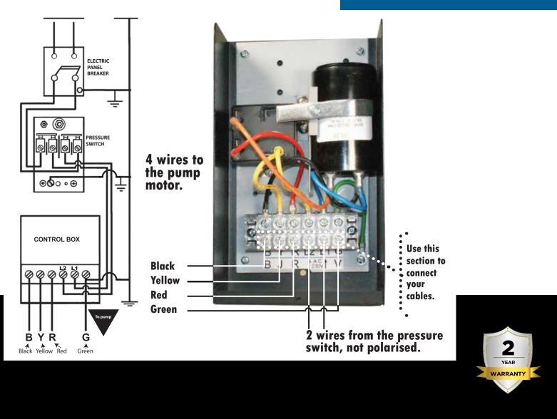
Suitable for three load wires and one ground wire deep well submersible pump motor.
